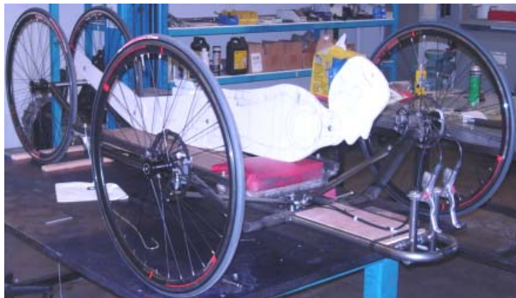
Gravity Racer ergonomics study during fabrication
